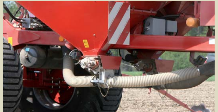
The metering devices are easily accessible from the sides of the hopper.
